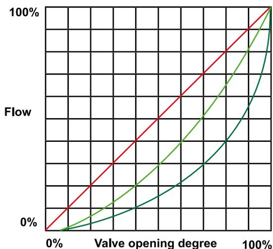
Fig. 1 Inherent flow characteristic at constant pressure drop
